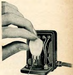
Be sure to line up index mark on bulb and socket
