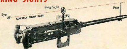
a Mk 13 ringsight and a Mk 7 post mounted on a cal. 30 B.A.M. gun.
