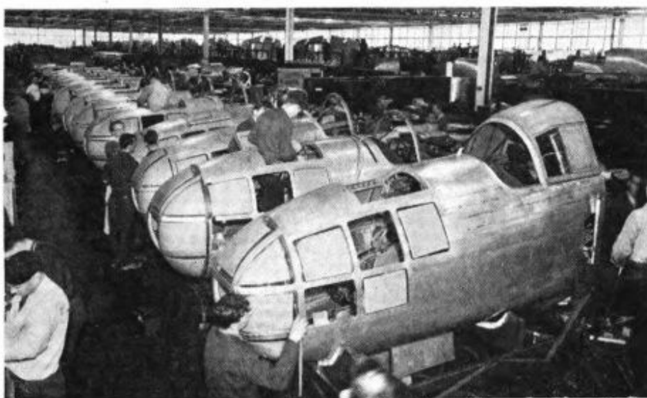
FIG. 35—FUSELAGE NOSE-SECTION ASSEMBLIES
