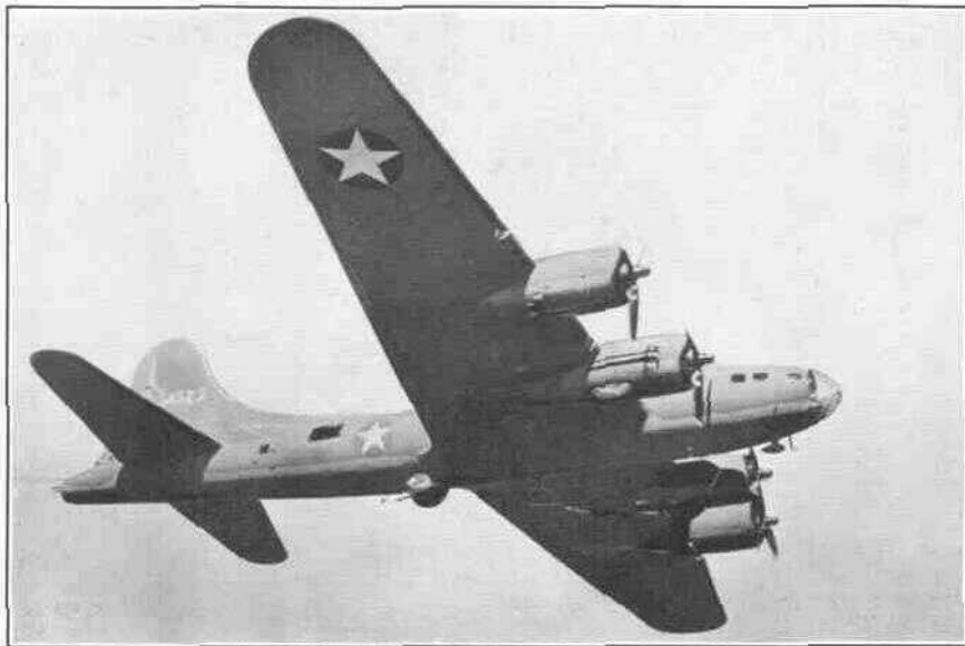
Photo. A1706. Boeing "Flying Fortress," showing ventral, and tail gun-turrets.
