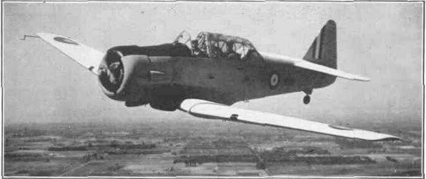
Photo. A1412. The North American "Harvard" has a 600 h.p. Pratt and Whitney "Wasp" radial air-cooled engine. The wings are tapered on leading-edge only.
