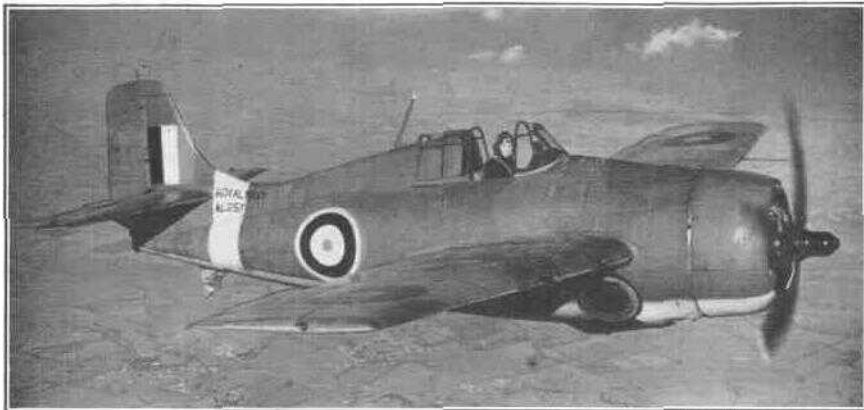
Photo. A 1281. The Grumman "Martlet," in use with the Fleet Air Arm, is a mid-wing monoplane. "AEROPLANE" Photograph
