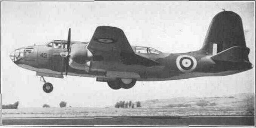
Photo. A1517. A Douglas "Boston" with its tricycle-type undercarriage in the act of retracting at take-off.
