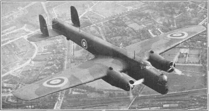
"AEROPLANE" Photograph Photo. A740. When the fins and rudders are placed inboard of the tips of the tail-plane, as in the Armstrong-Whitworth "Whitley," they are said to be inset.
