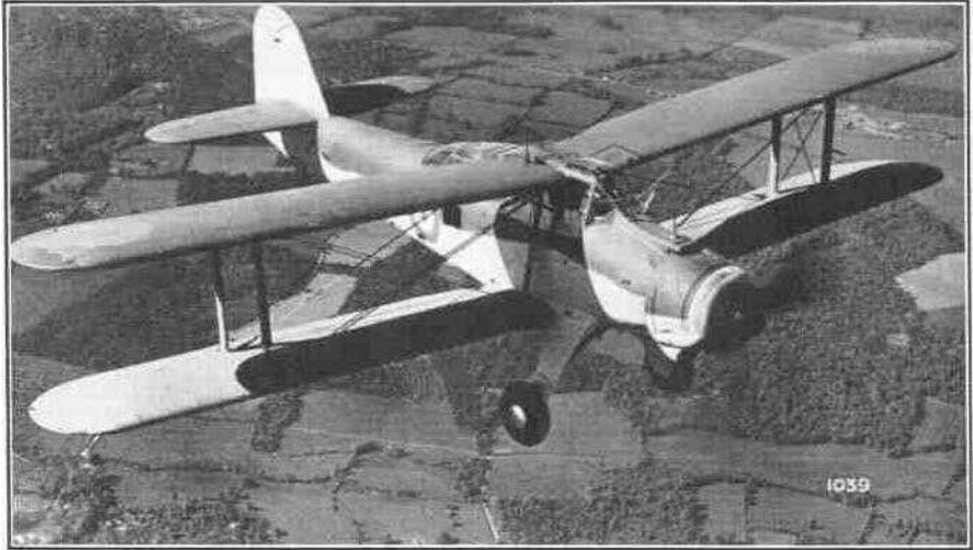
Photo. AI039. The Fairey "Albacore," a single bay Biplane, is used by the Fleet Air Arm for Torpedo attack.
