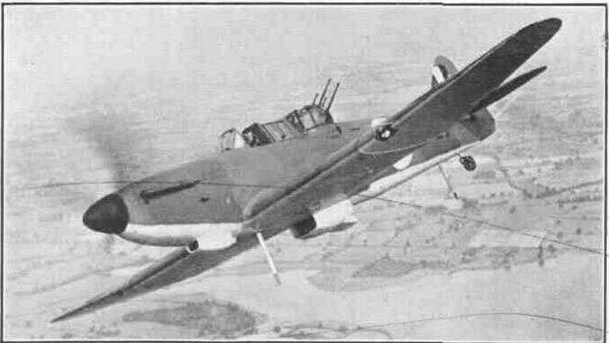
Photo. AI296. The gun-turret of the Boulton Paul "Defiant" is a special recognition point, for its glazed cop can be seen in either head-on or side view.
