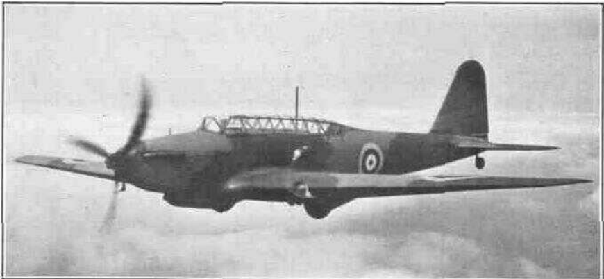
A16. The Fairey 'Battle' has a semi-retractable undercarriage. Note that wheels remain partially visible in flight.
