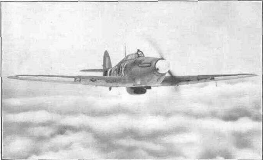
Photo. A1691. Hawker "Hurricane" showing radiator centrally placed beneath fuselage. "Aeroplane" Photograph
