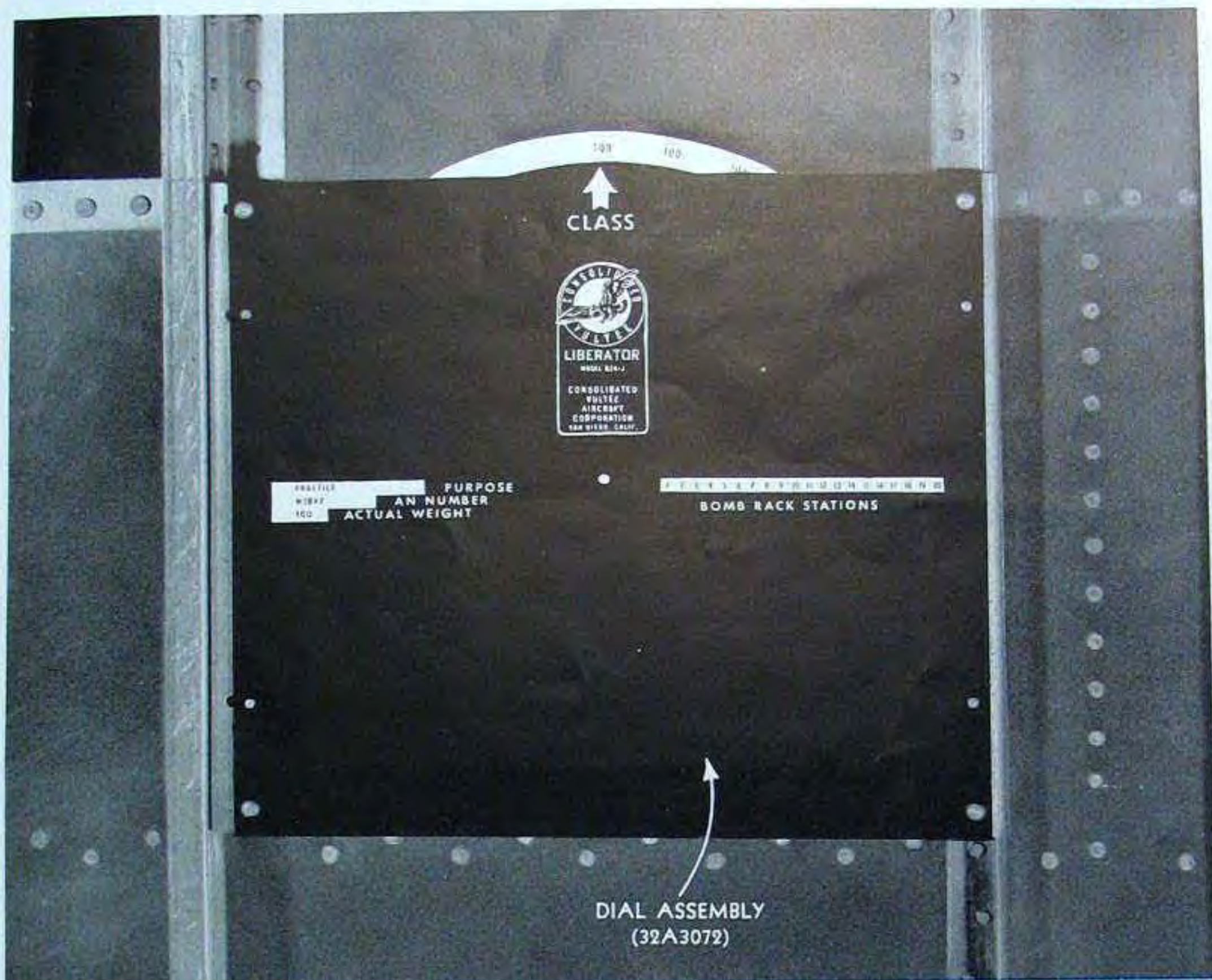
Figure 1. Bomb Loading Identification Placard Installed in Bomb Bay.
