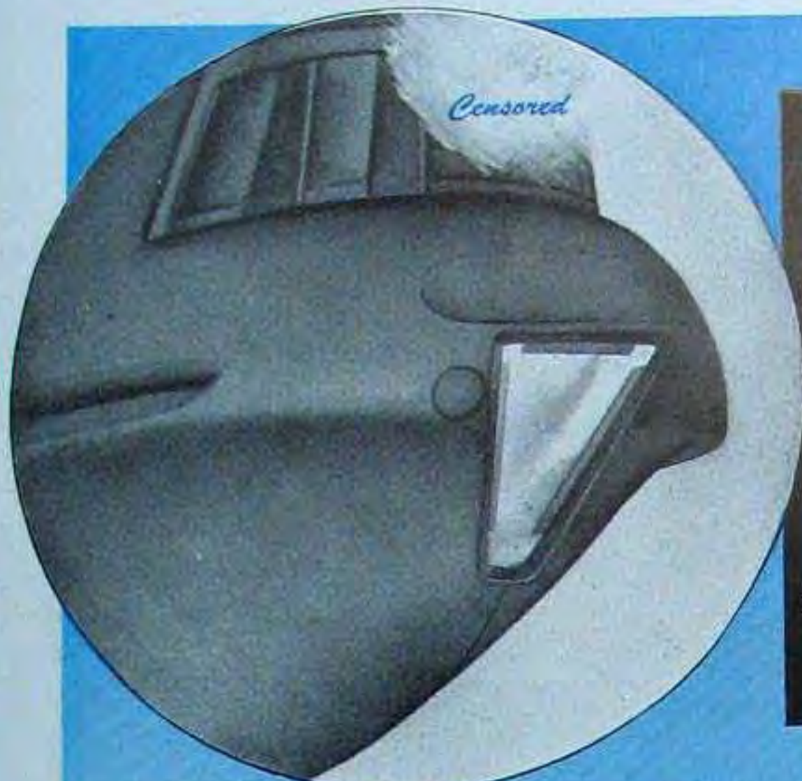
Figure 13. Redesigned Bombardier's Window Installed.
