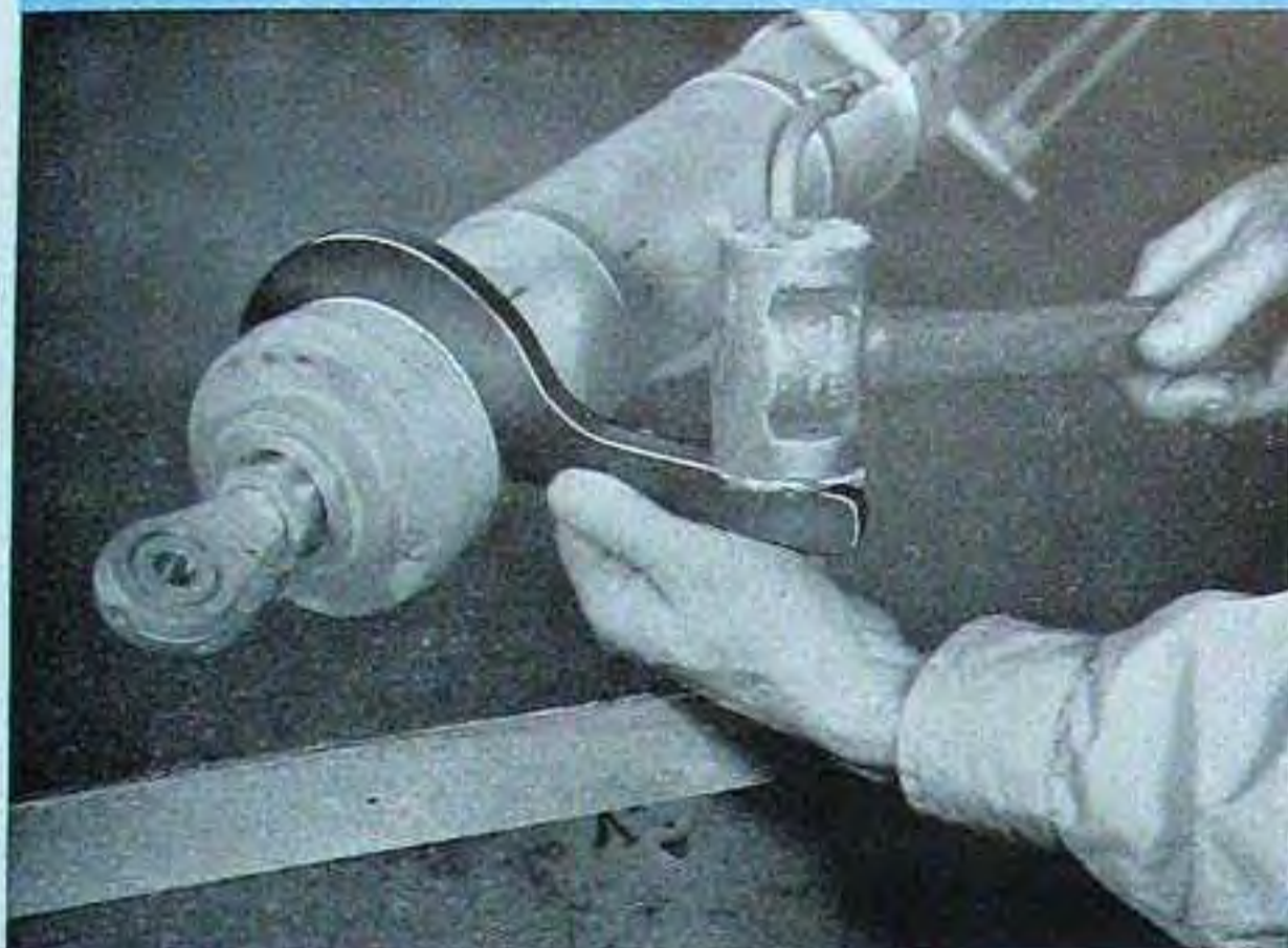
Figure 15. END CAP LOCKNUT WRENCH FOR MAIN LANDING GEAR CYLINDER (ST-00057)
