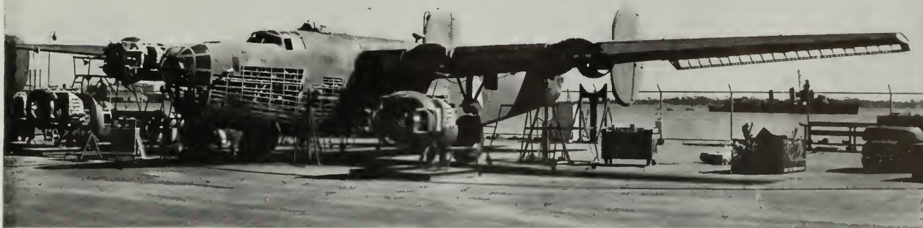
A B-24 Liberator, damaged in combat, is assigned to the Consolidated-Vultee School for training USAAF groundcrew mechanics at Camp Consair, San Diego. Part of the skin is removed, and only one engine is in place.
