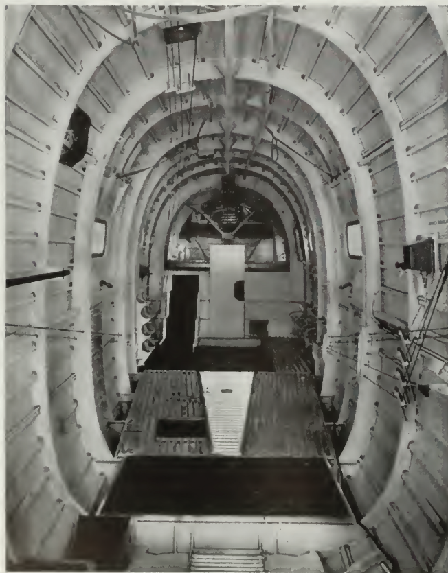
Operating controls are exposed, lines colored and parts stencilled to make instruction clear in this damaged B-24 at Camp Consair.
