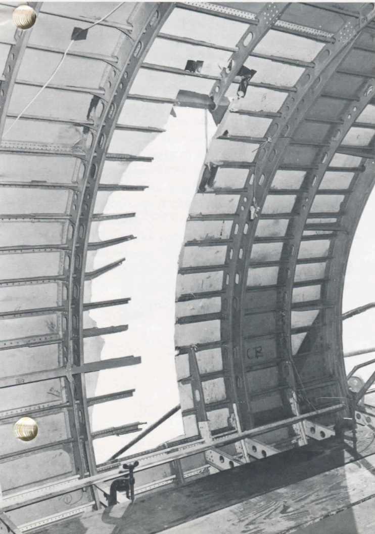
DAMAGE TO FUSELAGE SHOWING SPEAR ASSEMBLY IN FOREGROUND
