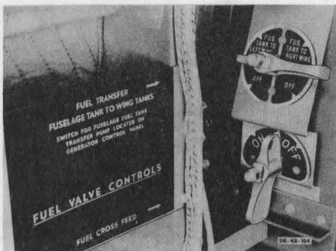
Figure 21—Fuel Transfer and Cross-feed Controls
