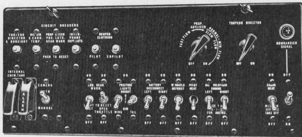
Figure 20—Pilot's Switch Panel
